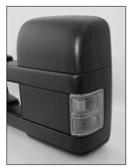
1. If the mirror's corresponding plug doesn't have pre-wired pins to power the turn signal and side marker, then you will need to use the included extension wires to hardwire these lights into their appropriate circuits using included wire taps.
